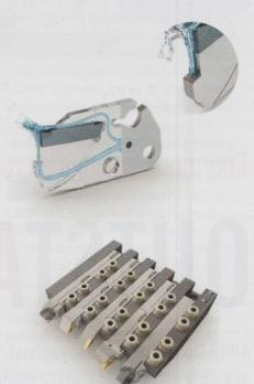
considerably reduced. Instead of having to lower cutting and feed rates to protect the tool, rates can even be increased. Productivity rises since tool life is significantly longer. Users report that their tools last up to three times longer or at least twice as long. Fewer tool changes ultimately relieves the work burden on operating personnel while significantly reducing machine down time
