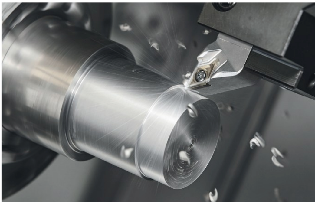
Bringing coolant directly to where it's needed: hybrid holder from Arno Werkzeuge, combining additive technology with conventional CNC milling
