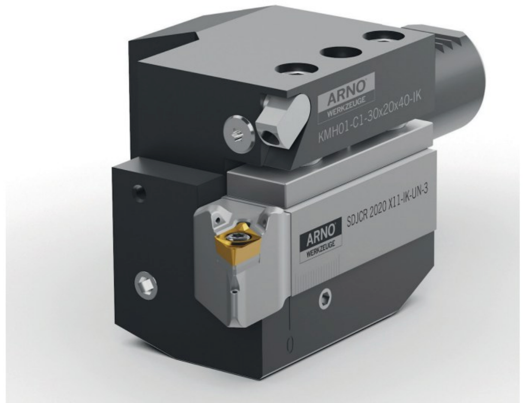
Clamp holders with internal coolant channels produced by hybrid processes at Arno, increase process reliability and improve surface quality in machining processes through optimised cooling
