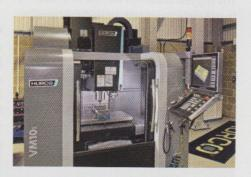
VMX line is the workhorse of 3-axis CNC machining centres, but Hurco does not stop at milling. The company works diligently to ensure its turning centres are up to par with its mills. The TMX, TMM, and TM lines include a range of turning centres with chuck sizes up to 25 inches and mill turn machines that support the done in one philosophy.
