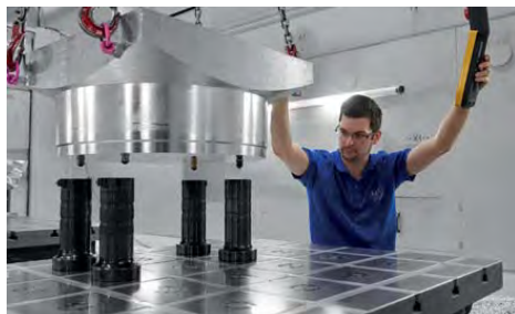
At MT Technologies, the workpiece is clamped in just a few simple steps for five-sided machining
