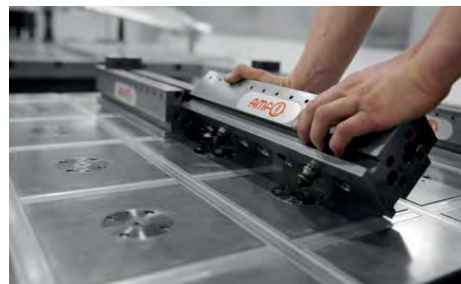
The zero-point clamping system is just as easy and logical as Lego
