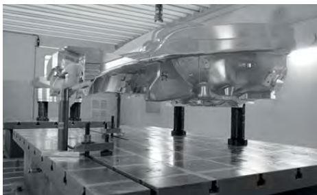
The clamping plates are equipped with K10 installation clamping modules from AMF at a grid pitch of 200mm
