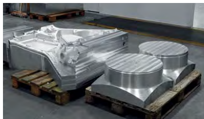
The side panel of the body and aluminium rims are machined from solid blocks
