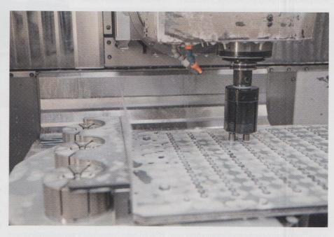
wear-free surface. On request, the manufacturer produces gripper inserts that are adapted to the workpieces. Blanks are also available, which customers can adapt individually for their application. With the new gripper, AMF is expanding its programme for automating machine tools, which already includes zero-point clamping technology, a collet chuck and a similarly interchangeable cleaning tool.
