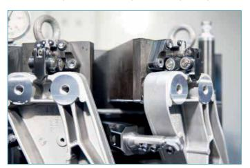
change of fixtures to maintain a high level of machine utilisation, particularly at the start-up phase of a new product."
