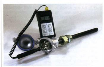
in the course of the DIN ISO 9000 ff (e.g. at heat-treating furnaces). The thermocouple in a testable design will be supplied as a single or double exchangeable measuring insert. The terminal block has a centre hole which enables
