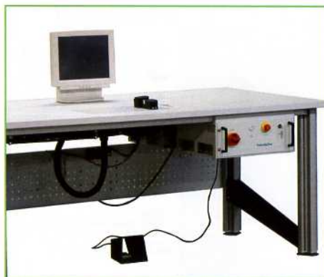
Telso-Splice TST 50205 ultrasonic desktop strand welding device from the specialists Telsonic AG, Bronschhofen
