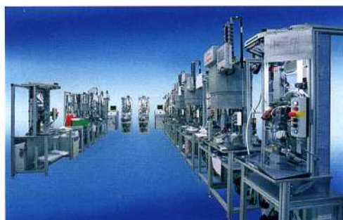
For the new and as yet unique urea injection technology for car diesel engines, ZELTWANGER developed and built a semi-automated manual production line with 18 stations for the world's biggest automotive parts supplier, Bosch.
