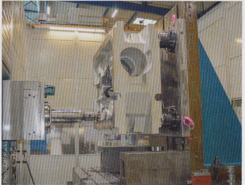
On the huge Union drilling installation for heavy machining, AMF's extra-strong K40-H modules are used for direct clamping of the workpiece.
