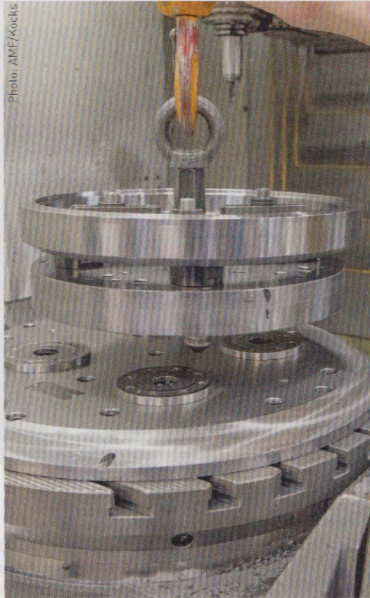
Because re-clamping is so simple with AMF neutral-point clamping, there is no problem inserting unplanned replacement parts requiring immediate manufacture into the production sequence.
