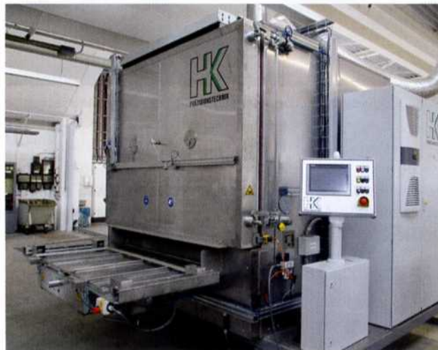
Circulating hot air oven for hot forming of planar and pre-formed composite semi-finished products
