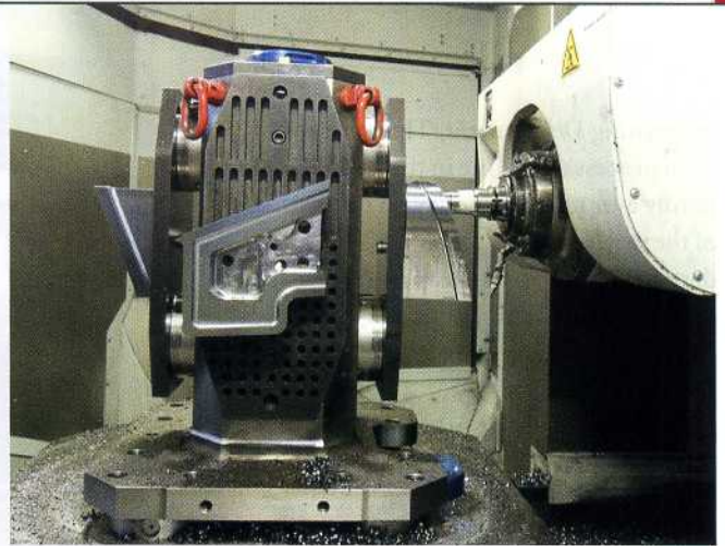
3 GF Machining Solutions adjusted the two Mikron HPM 1350U centres to work with the dry milling method customary at BMW
