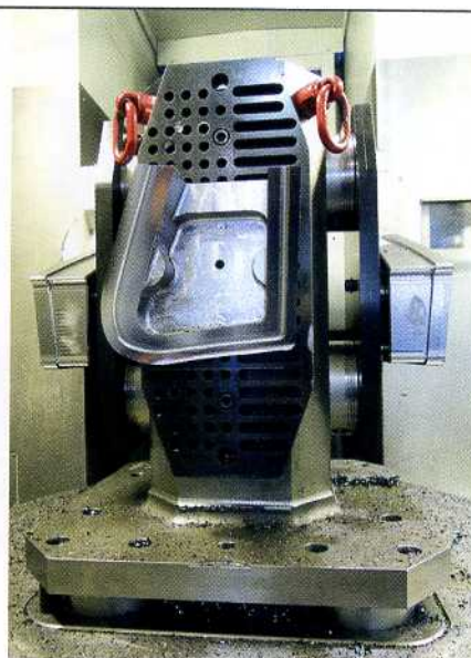
4 The use of tombstones in the Mikron machines is part of the toolmaking optimization spectrum at BMW Munich
