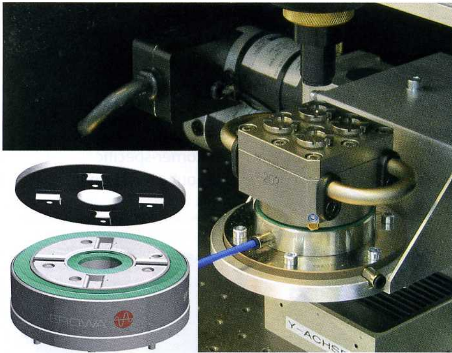
The Fine Tooling System is a clamping chuck for small dimensions.
