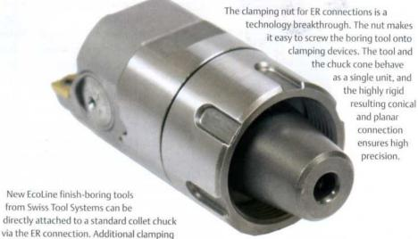
The ER connection allows users of the boring tool to save on tooling costs by eliminating the need for a master shank and for extensions or reductions. According to Swiss Tool Systems, the breakthrough clamping concept, which includes a chuck cone grip and face contact, delivers very good rotational accuracy, maximum rigidity and a very strong retention force. Collet chucks that have an ER connection as specified in DIN 6499 are commonly used in mechanical workshops around the world.
