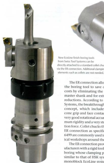
wiss Tool Systems AG has intro-Oduced the EcoLine finish-boring tool, an innovative development that includes a built-in ER connection which enables the tool to be directly attached to an ER collet chuck. This, says the manufacturer, is a world first.
